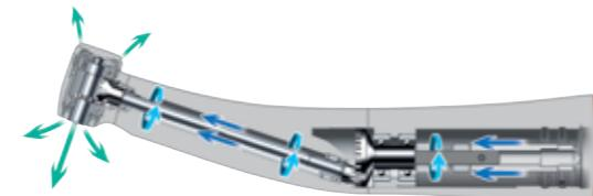
Low-speed handpieces incorporate gearing systems that require extra solution penetration. The NSK rotation system guarantees optimum oil delivery to the internal components of all low-speed handpieces.
